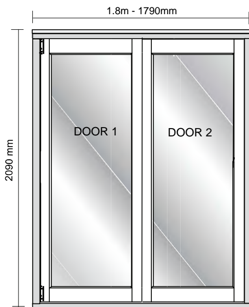
Shows left opening door set
