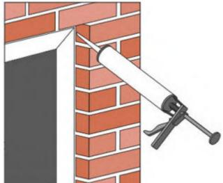
Ensure the frame is free from dust and debris before applying to ensure an adequate barrier is created to prevent any water or air leakage. Remove any protective film before sealing.
