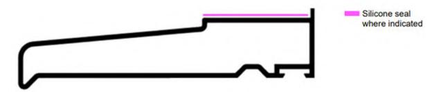
Carefully lift the window and fit it into the brickwork opening, resting on the cill and bed of silicone.
