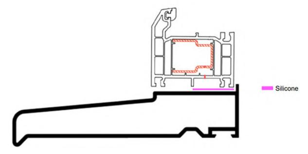
**IMPORTANT:** The frame should not be pushed tight back to the plaster line as this can lead to the door being fitted in twist.
