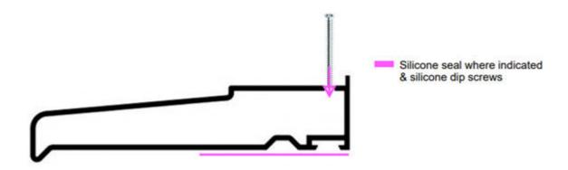
If preferred, the cill can be fitted to the frame before the whole unit is fitted into the opening. The cill will require screwing to the frame jambs and window profile (screws not supplied) from the underneath and appropriately sealed.
