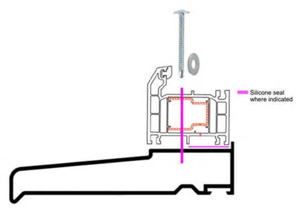
**VERY IMPORTANT:** When all the fixing points are secured, carefully check the frame is tightly fixed together and is square. Diagonals of the frame must be equal. Do not proceed with installation if the frame is not square and level on all planes.
