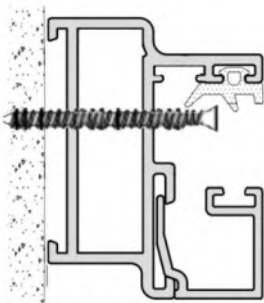
Fixing point through sidelights
