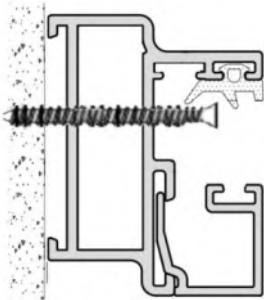
Fixing point through sidelights
